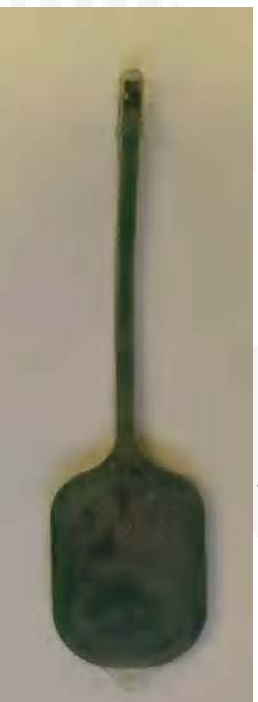
Intracranial pressure sensor implant with Diamond Like Coating (DLC)
